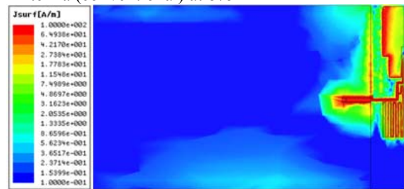
Figure 4-2 Current distribution of a penta-band Metamaterial Antenna at 875 MHz
